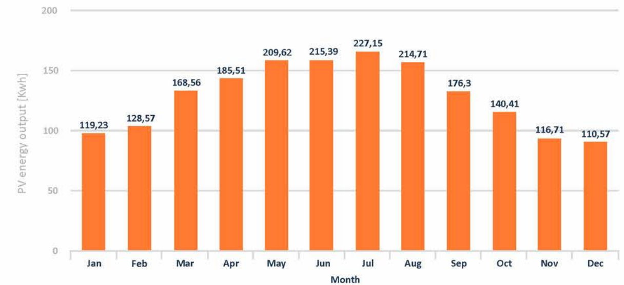
Monthly energy output from fix-angle PV system
