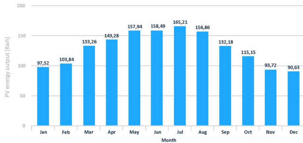
Monthly energy output from fix-angle PV system
